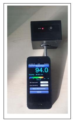
When the calibrator is on, Press "Calibrate"
